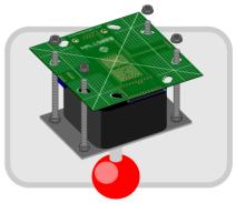
STEP 5 Attach a Joystick extension cable to the 9 pin D connector and plug the stick into Port B for **CALIBRATION**.
